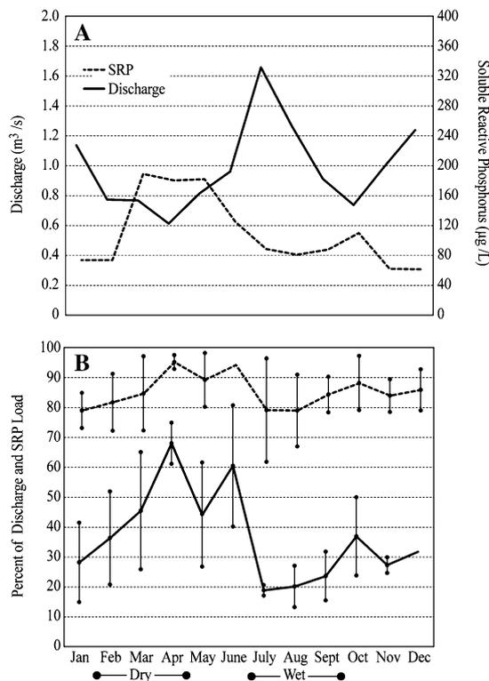
**Fig. 5** **(A)** Mean monthly discharge and SRP concentration at Lower Salto 30 (1997–2001) and **(B)** Proportional contribution of discharge and SRP load (monthly mean  $\pm$  s.d., 1997–2002) by high-SRP geothermal springs and swamp-forest
