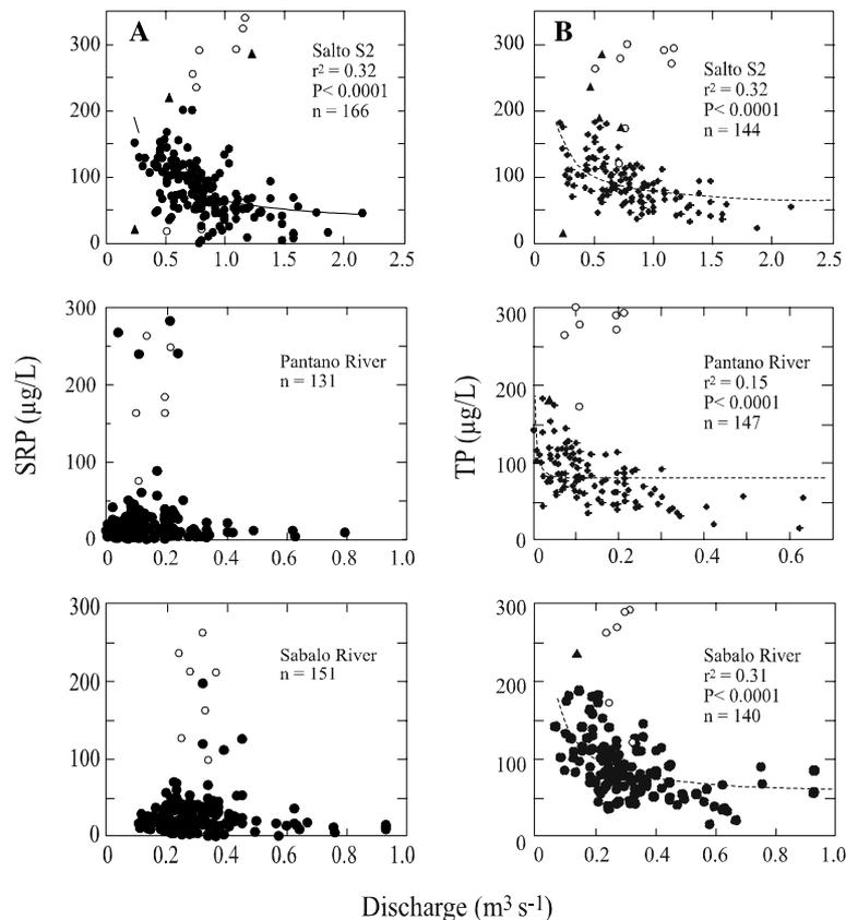
**Fig. 3** Plots of (A) SRP and (B) TP concentration vs. discharge for the Lower Salto (S2), Pantano, and Sabalo Rivers. Dashed lines are best fit regression relationships between concentration and the inverse of discharge. Open circles are ENSO related data, closed triangles are rejected outliers. Fitted line formulae were determined by linear
